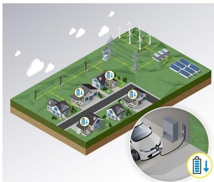
When the energy supply is lower than the demand, vehicle charging stops.
